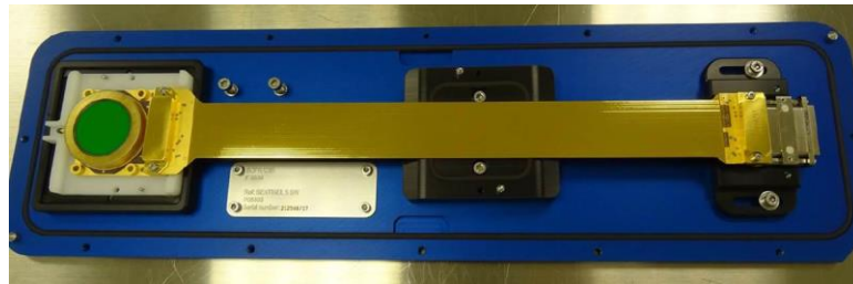
Figure 2-6 : NGP sensor in Sentinel-5 detector package
